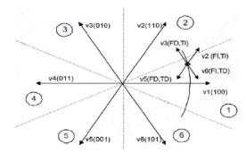
Fig-1: Stator flux vector locus
