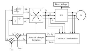
Fig.1 Block diagram of DTC scheme
